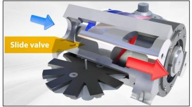
To obtain the best possible efficiency at every working condition, Daikin compressors can adjust the geometry of the discharge port according to the real operating conditions slightly delaying or anticipating the discharge phase of the refrigerant minimizing the losses for under or over compression and so enhancing the efficiency. This is possible thanks to a sliding valve.
