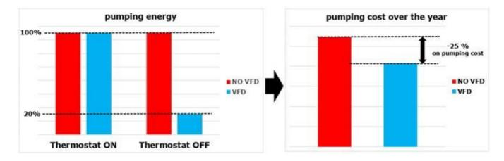
Thanks to the saving on pumping cost, the payback time for the Inverter Kit is approximately one year.
