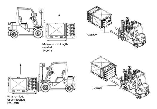
Fig. 46 – Indications for stacked units installation
