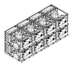
Fig. 42 – Pump module installation
