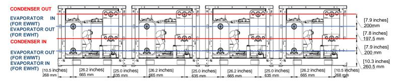
When pump module is not equipped, the customer can connect the plant water piping indifferently to the left or right side of the manifold modules system. When pump module is supplied, the water connection can only be done to the pump suction pipe.
