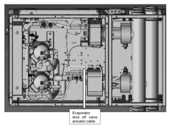
Fig. 36 – Evaporator shut off valve actuator cable routing
