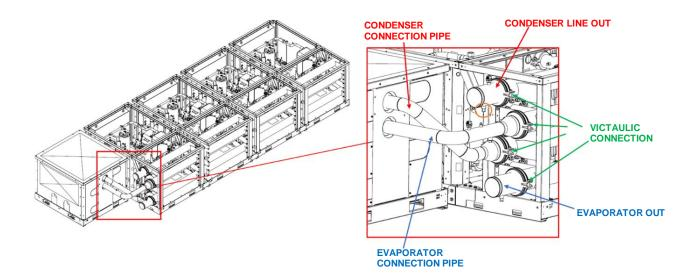
The pump module can be installed only on one side of the unit- manifold system. The water inlet installation is constrained to the pump suction.
