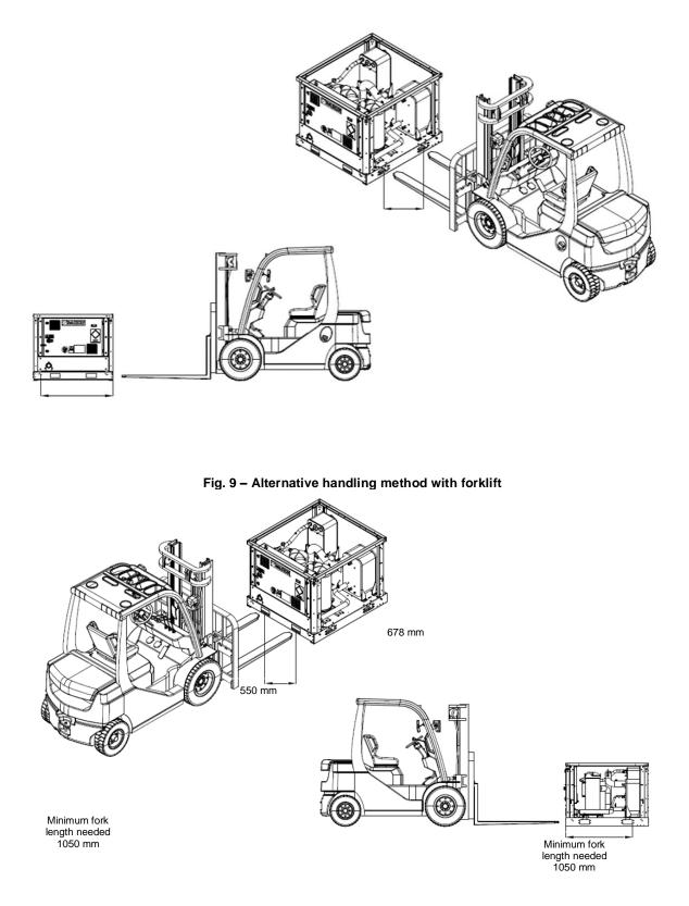
Fig. 10 – Alternative handling method with pallet truck
