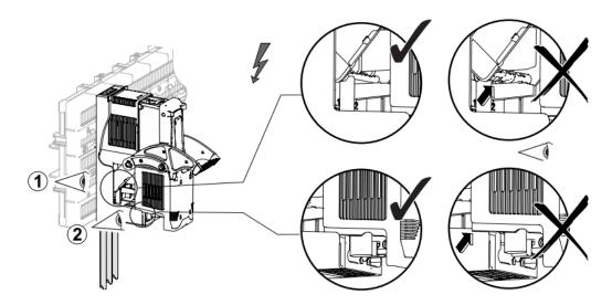
4) Insert the mobile part of the fuse holder in to the fixed one, being careful not to damage the part.
