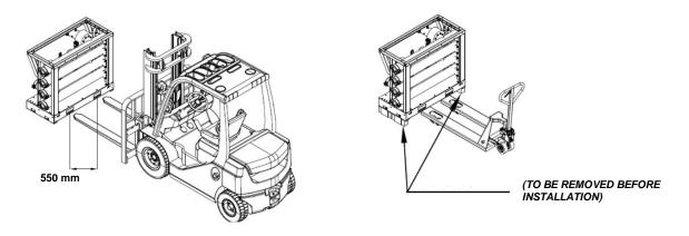
The module consists of the unit and the manifold connected; it can be lifted by forklift. Only the base frame holes must be used to lift the module.
