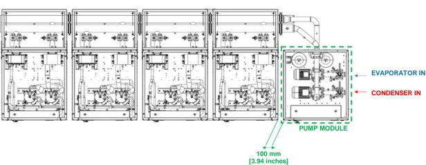
Fig. 43 – Pump module installation – piping details
