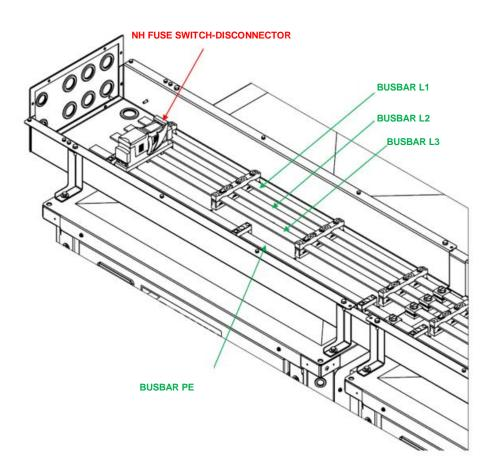
The electrical connection of the units to the power bar system is done through a multipolar cable, 3 phases with ground. The three phases shall be connected to the fuse holder, equipped with each module, and the ground (PE) shall be connected to the ground bar (Busbar PE).
