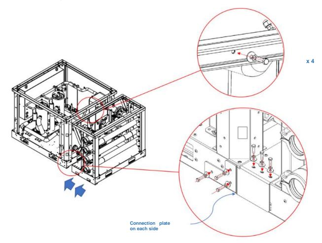
After installation of manifold module and before connection to the chiller module, it is important to clean and remove welding oxides and other contamination products deriving during production of the water piping. The cleaning steps are the following:
