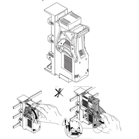
Fig. 58 – NH fuse switch disconnector
