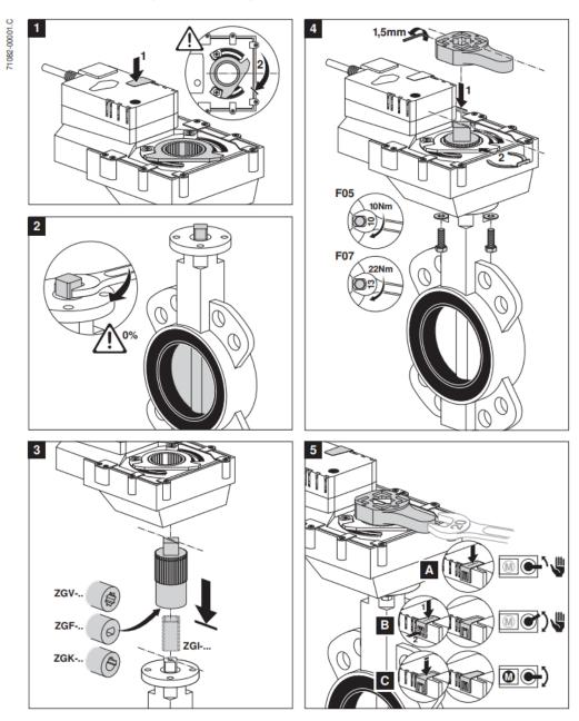
Fig. 29 – Mounting instructions for valve actuator
