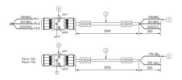
Fig. 35 - Shut off valve actuator wiring diagram
