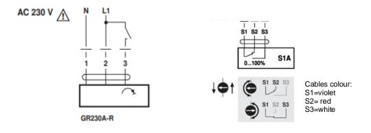
Fig. 33 - Cable adapters for evaporator shut off valve actuator and limit switches
