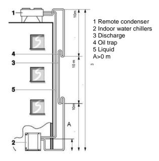
piping length: equivalent = 50 m maximum height = 30 m
