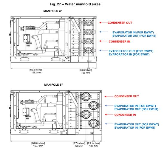
EWWT-Q and EWLT-Q series are equipped with heat exchangers that need to work all counter-current. In these cases, the water inlet for evaporator is on the top pipe and the water inlet for condenser is on the bottom pipe.
