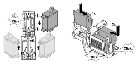
3)Insert the fuses into the body exerting a slight pressure downwards for the single fuse, and a slight pressure upwards for the pair of fuses: in this way the fuses are hooked.
