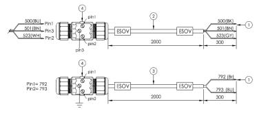
Fig. 34 - Cable adapters for condenser shut off valve actuator and limit switches
