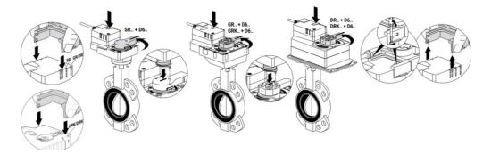
The valve shall be mounted on the unit following the indications in figure below.
