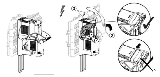
5)Push the lever of the fuse holder upwards; the mobile part is hooked and slides inwards. 6)Apply power supply to the duct
