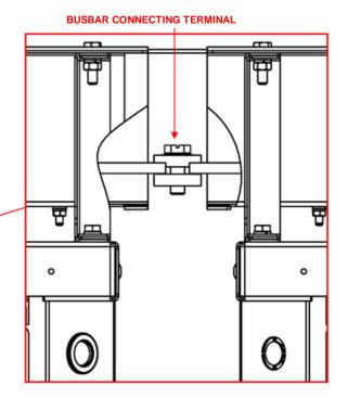
Top view of the open power bar module
